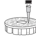
1. Fill the disk using slow, even pressure. The sample water will fill the spaces between the baffles in a counterclockwise order. Each space will fill from the bottom to the top. Sample water should be added until the sample water in the fourth chamber fills **to the top** of the chamber slightly past the embossed fill line. It is OK to fill slightly past the fill line.
