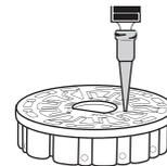
1. Fill any unused section of the disk using slow, even pressure. Add the sample water until the Blank Chamber is full and the Over Flow Chamber is partially filled.
