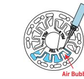
5. Wet disks should be dried thoroughly with a lint free wipe. Handle the disk by the edges. Between tests store the disk on a flat surface. Do not agitate a partially filled disk to avoid leaking and contamination. Partially used disks should be discarded at the end of the day.
