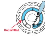
4. Do not introduce air bubbles into the disk. The reagent chambers will not fill entirely and results will be inaccurate. As soon as a bubble starts to form, pull back on the plunger to draw the bubble out of the disk. Begin the filling process again.
