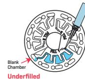
4. Do not introduce air bubbles into the disk. The reagent chambers will not fill entirely and results will be inaccurate. As soon as a bubble starts to form, pull back on the plunger to draw the bubble out of the disk. Begin the filling process again.
