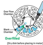
3. Do not under fill the disk. If the disk is under filled, the blank chamber will not be full. The reagent chambers will not fill entirely and results will be inaccurate.
