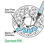
2. Do not overfill the disk. If the disk is overfilled, sample water will flow out of the vent hole in the center of the disk. The disk is not leaking. Dry the disk and run the test.
